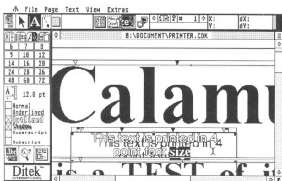
■ The fonts are mathematically created from within Calamus so that at the larger sizes they are still perfectly shaped.
