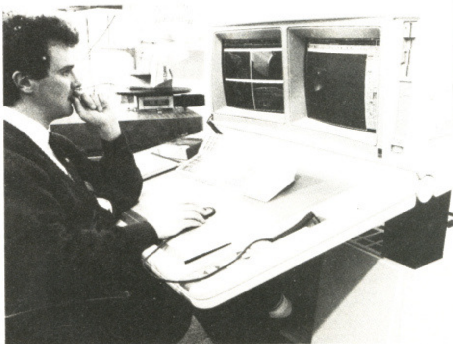
▲ The ultimate in workstations. The large screens are virtually a necessity for many of today's CAD applications. The graphics tablet offers the perfect inputting device with output being sent to a plotter later.
